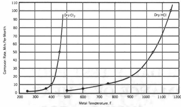
**FIG. 2 CORROSION OF CARBON STEEL IN CHLORINE AND HYDROGEN CHLORIDE**
