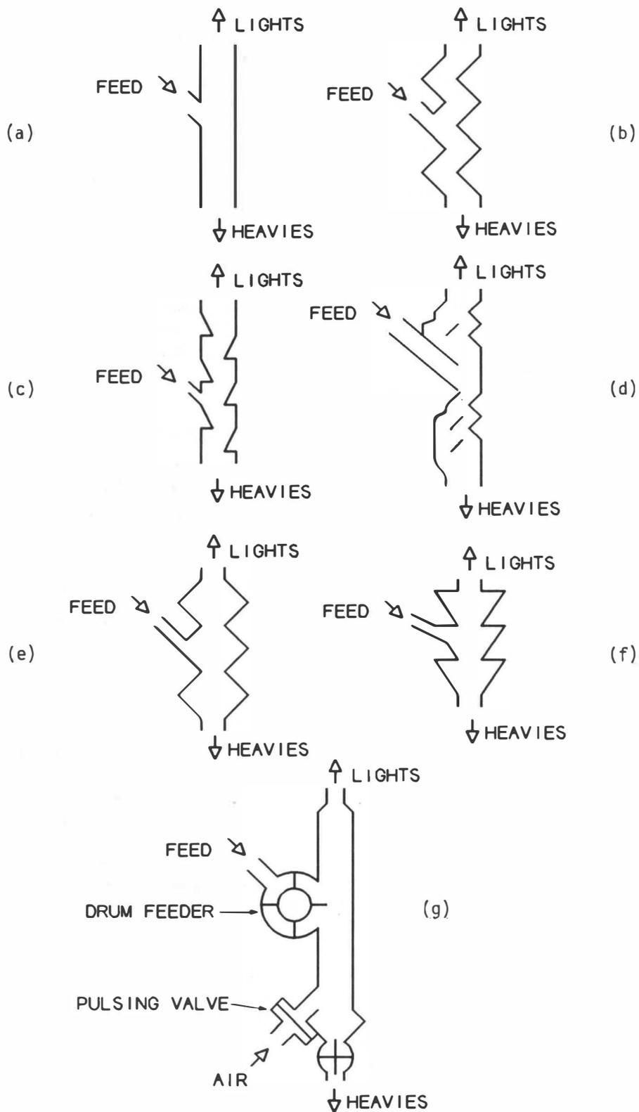
FIG. 4 CHRONOLOGICAL PROGRESSION OF VERTICAL AIR CLASSIFIERS: (a) STRAIGHT; (b) ZIG-ZAG; (c) UTAH THROAT; (d) DUKE THROAT; (e) ZAG-ZAG; (f) STACKED TRIANGLE; (g) ACTIVE PULSED-FLOW [17]
