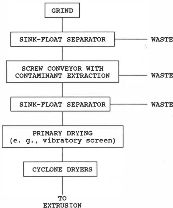
FIG. 2 FLOW DIAGRAM FOR THE FILM WASHING SEGMENT OF THE INTERNATIONAL PLASTICS ITALIANA LOW-DENSITY POLYETHYLENE RECOVERY OPERATION [13]
