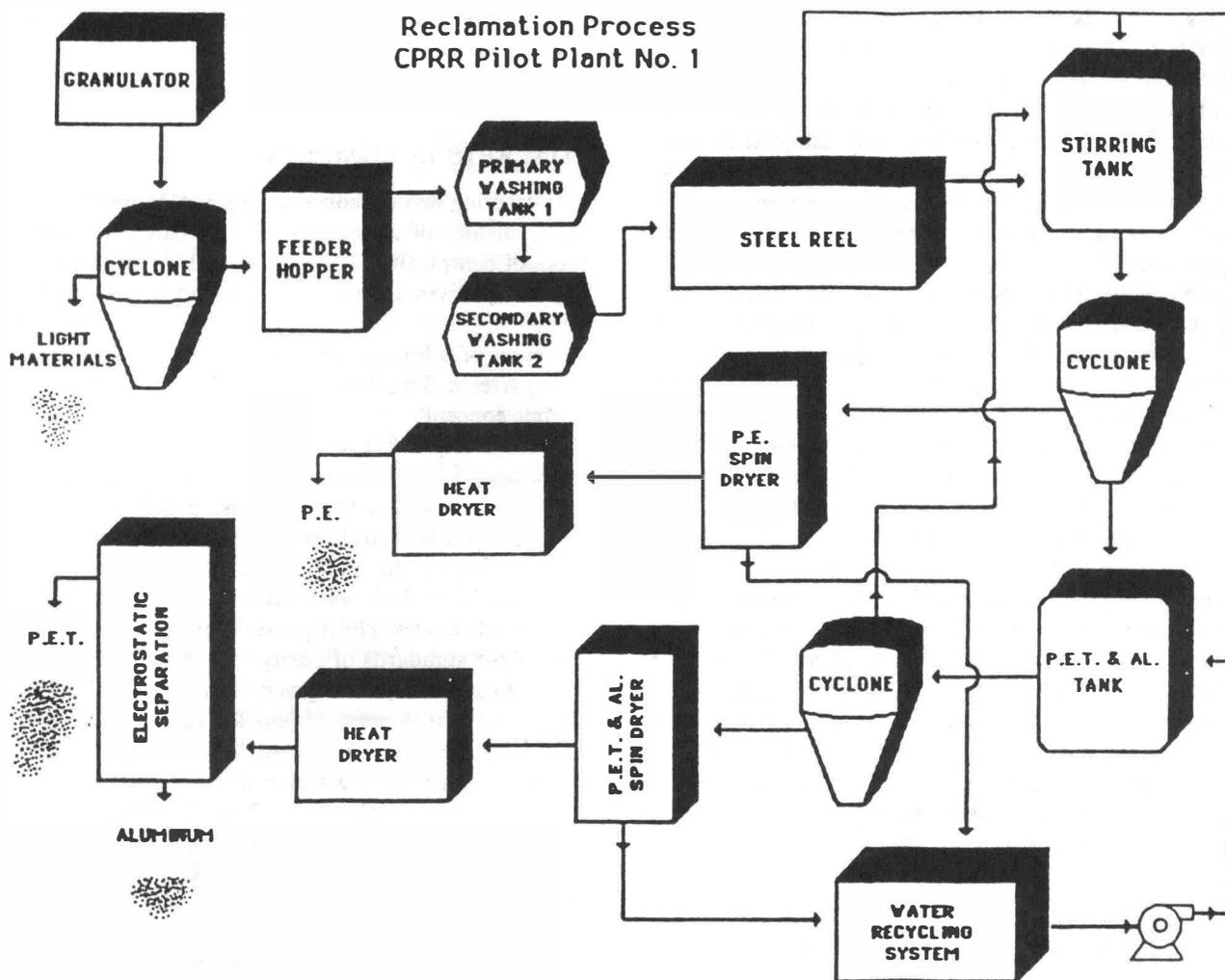
FIG. 1 FLOW DIAGRAM OF THE CENTER FOR PLASTICS RECYCLING RESEARCH PROCESS TRAIN TO RECOVER PLASTICS FROM CONTAINERS [12]
