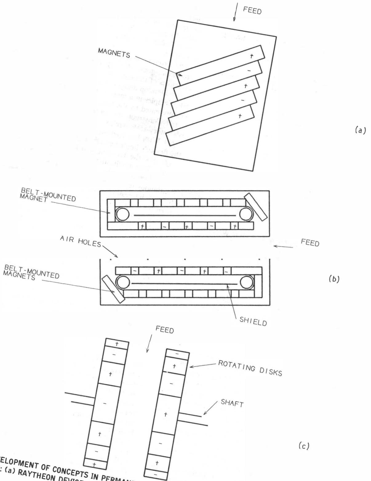
FIG. 3 DEVELOPMENT OF CONCEPTS IN PERMANENT-MAGNET EDDY-CURRENT NONFERROUS METAL SEPARATORS: (a) RAYTHEON DEVICE SHOWN FROM ABOVE; (b) CUTAWAY OF DOUBLE BELT-MOUNTED AIR TABLE DEVICE; (c) DELFT UNIVERSITY DEVICE [16]
