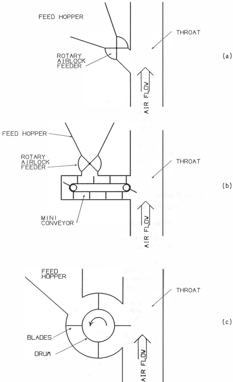
**Fig. 5 DEVELOPMENT OF A FEEDER SYSTEM FOR AIR CLASSIFIERS: (a) ORIGINAL ROTARY AIRLOCK FEEDER; (b) ADDITION OF A MINI-CONVEYOR, ALLOWING OPTIMAL ORIENTATION OF THE ROTARY AIRLOCK AND ELIMINATION OF RAMP; (c) ROTARY DRUM FEEDER, OFFERING THE ADVANTAGES OF MINI-CONVEYOR SYSTEM WITH GREATER SIMPLICITY**
