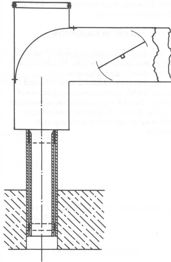
FIG. 3 MODIFICATION OF 4-INCH-DIAMETER NOZZLE WITH 3-INCH PIPE SLEEVE
