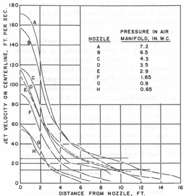
FIG 1 TYPICAL VELOCITIES IN AIR JETS FROM 4-INCH DIAMETER NOZZLES
