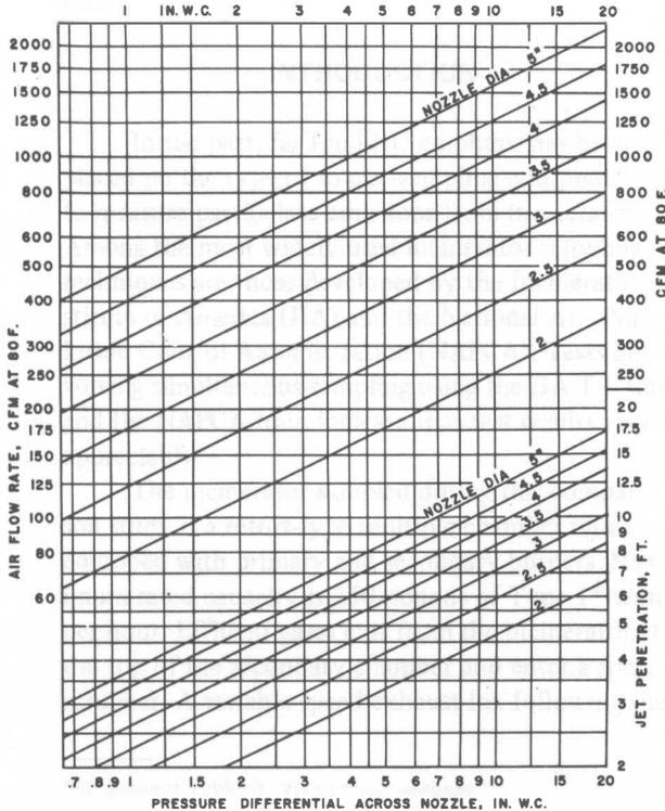
FIG. 2 AIR FLOW AND JET PENETRATIONS AT 1500 FPM AS FUNCTIONS OF NOZZLE DIAMETER AND PRESSURE DIFFERENTIAL
