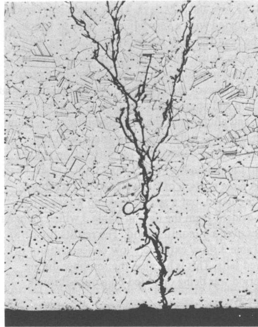
FIG. 5. STRESS-CORROSION CRACK IN C-RING OF TYPE 310 STAINLESS STEEL EXPOSED TO INCINERATOR DEPOSIT UNDER HUMID CONDITIONS (100 X)
