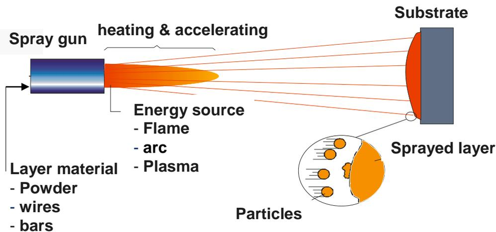
Figure 1 Thermal Spraying - Principle
