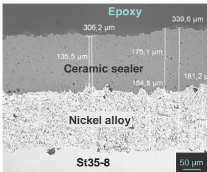
Figure 6a layer system as sprayed
