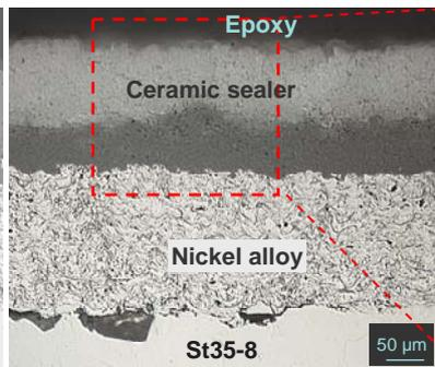
Figure 6a Layer system after use (500h, 540°C)
