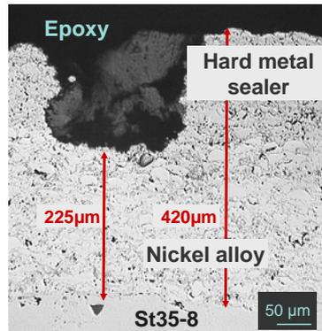
Figure 5b corrosion of the sealer (700h, 430°C)
