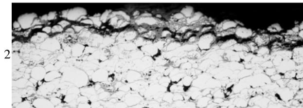
Figure 3a Layer shaped corrosion, partially flaking of corrosion products (substrate 15Mo3, exposure temperature 430°C, exposure time 470h)
