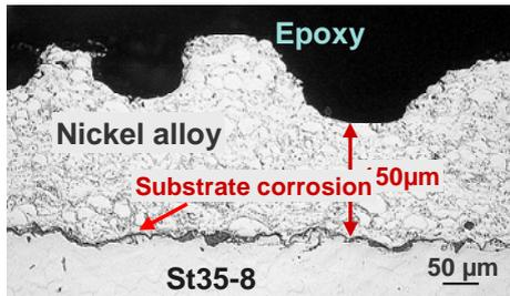
Figure 5a corrosion of the Nickel alloy (670h, 350°C)
