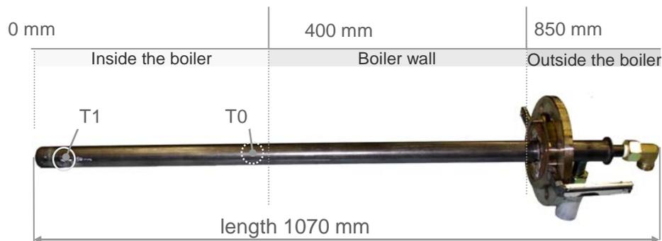
Figure 4 material probe
