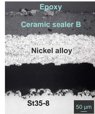
Figure 5c Flaking of the layer system (500h, 430°C)
