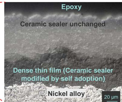
Figure 6a Detail view formation of a dense thin film between ceramic and nickel alloy
