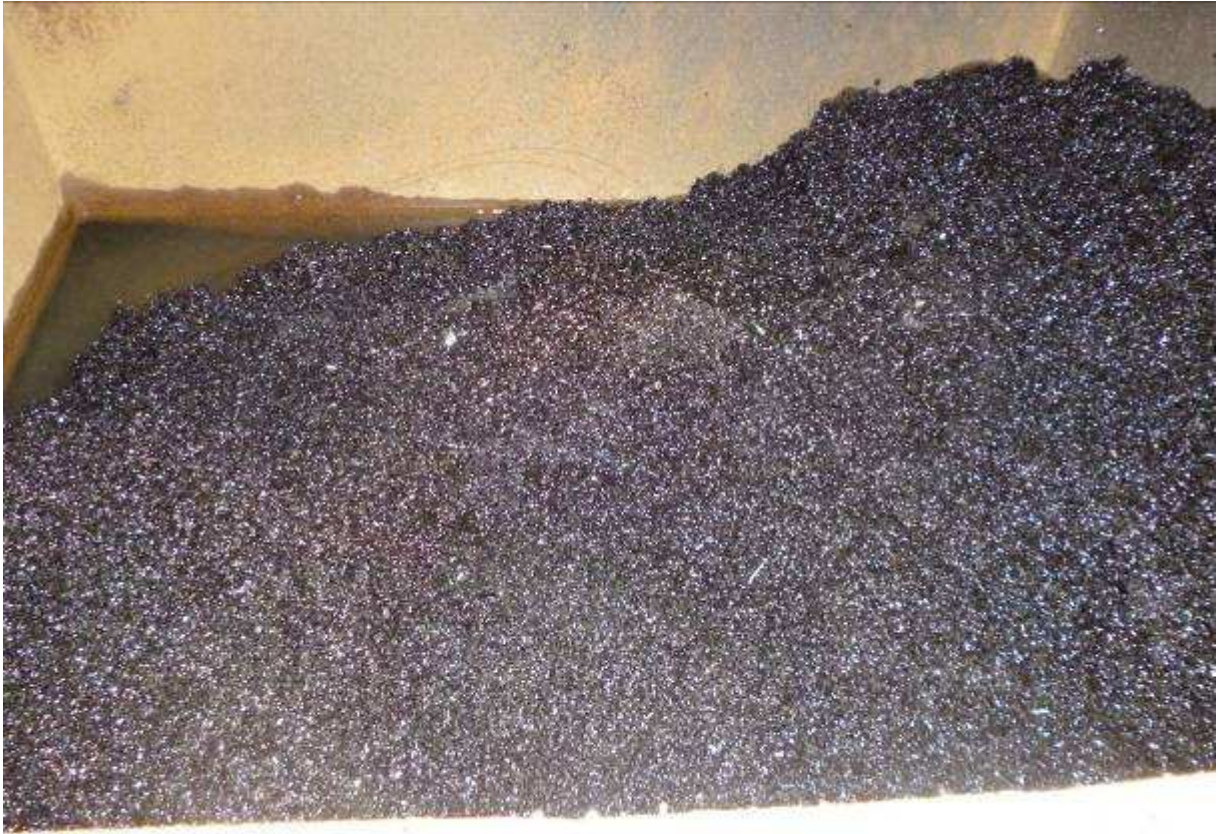
Picture 11. Vitrificated ash at PVG GS Platech Plant
