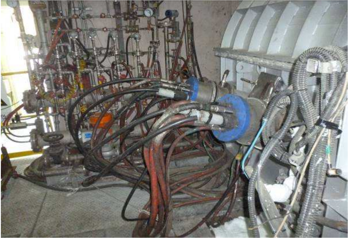
Picture 9. Plasma torches at PVG GS Platech Plant
