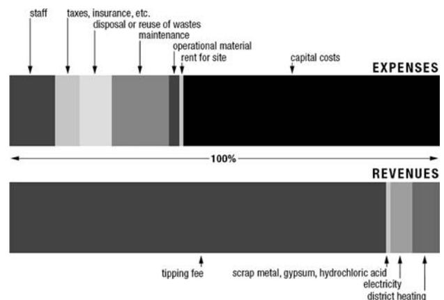
**Fig. 6** Expenses and revenues of a German waste-to-energy (WTE) facility
