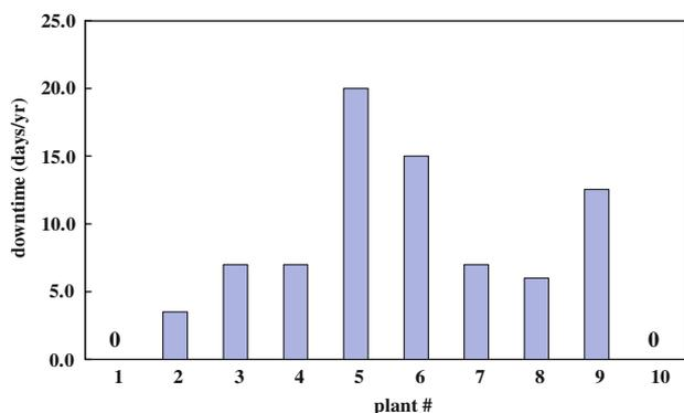
**Fig. 3** Non-scheduled downtime due to corrosion of waste-to-energy (WTE) plants (A1, B1, etc. refer to different waste-to-energy (WTE) facilities responding to the WTERT survey)
