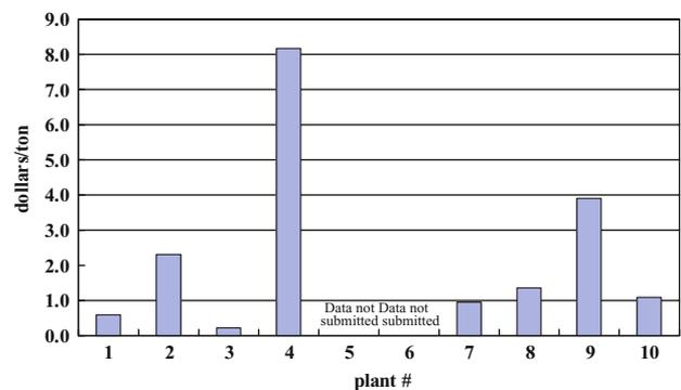
**Fig. 5** Cost due to corrosion per ton of MSW combusted (A1, B1, etc. refer to different waste-to-energy (WTE) facilities responding to the WTERT survey)
