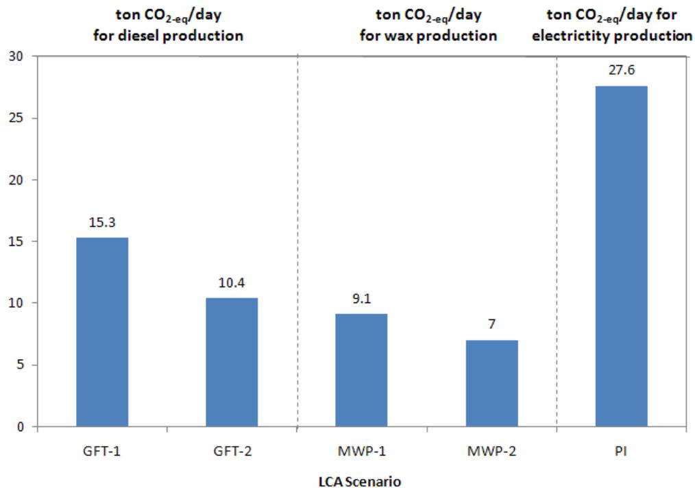
**Figure 5.5.** Comparison of Estimated Greenhouse Gas (GHG) emissions in terms of ton of CO<sub>2</sub>-eq per day of operation with the feed rate of 20 metric tons of waste plastics
