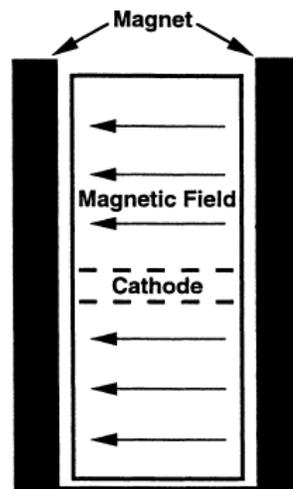
**Figure 4.2.** Schematic of Magnetron Microwave Tube [Adapted from Thostenson et al 1999]
