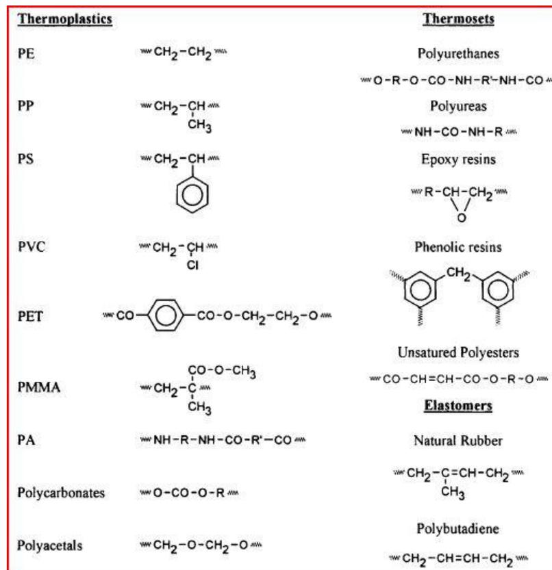
**Figure 1.3.** Examples of Thermoplastics and Thermosets
