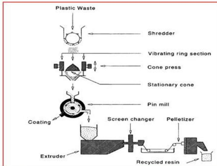
**Figure 2.1.** Typical Reclamation Process of Plastic Recycling [Adapted from Aguado 1999]
