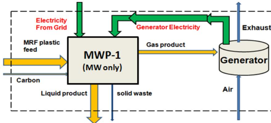
**Figure 5.2.** Material and energy flows of the MWP-1 process
