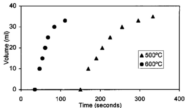
**Figure 4.5.** Cumulative Yield of Products for MWP of 50 grams of HDPE Over Time at 500 °C and 600 °C. [Adapted from Ludlow-Palafox (2001)]
