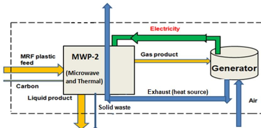
**Figure 5.3.** Material and energy flows of the MWP-2 process
