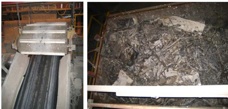
**Figure 4:** Left: Overhead electromagnets recover ferrous scrap from the bottom ash; Right: Recovered ferrous scrap
