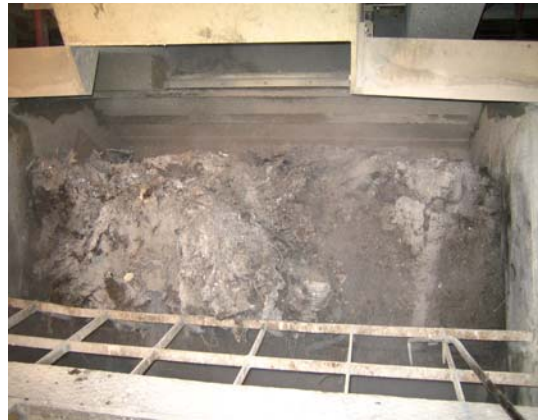
Figure 3: Back-end of the bottom ash quench from where the ash is conveyed to the magnetic separation
