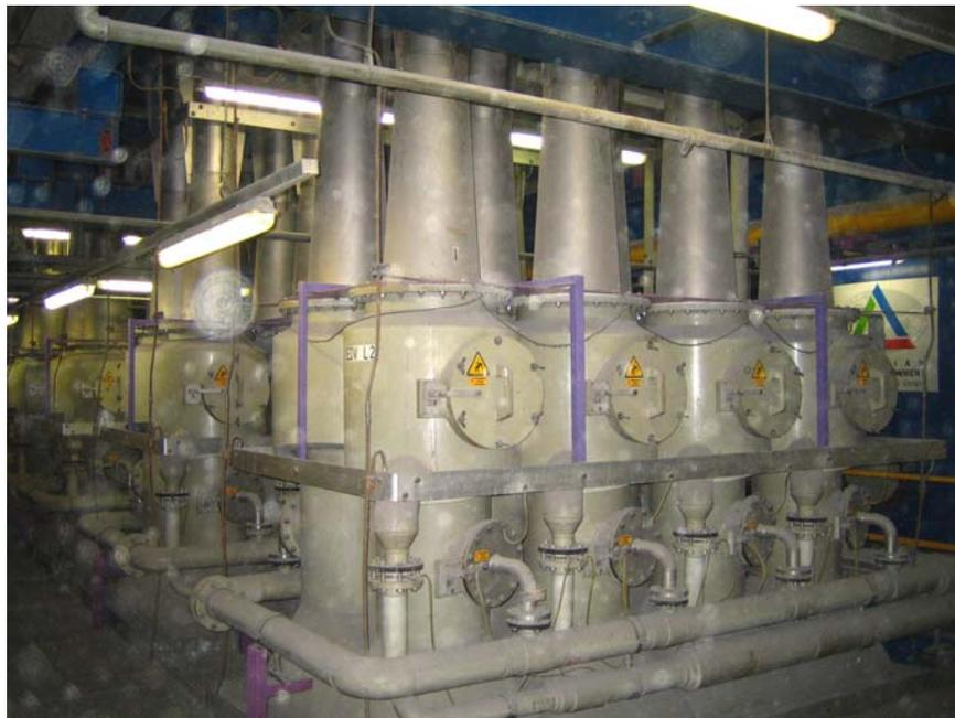
**Figure 8:** Electrodynamic venturi reduces the dust content to < 1mg/nm<sup>3</sup>
