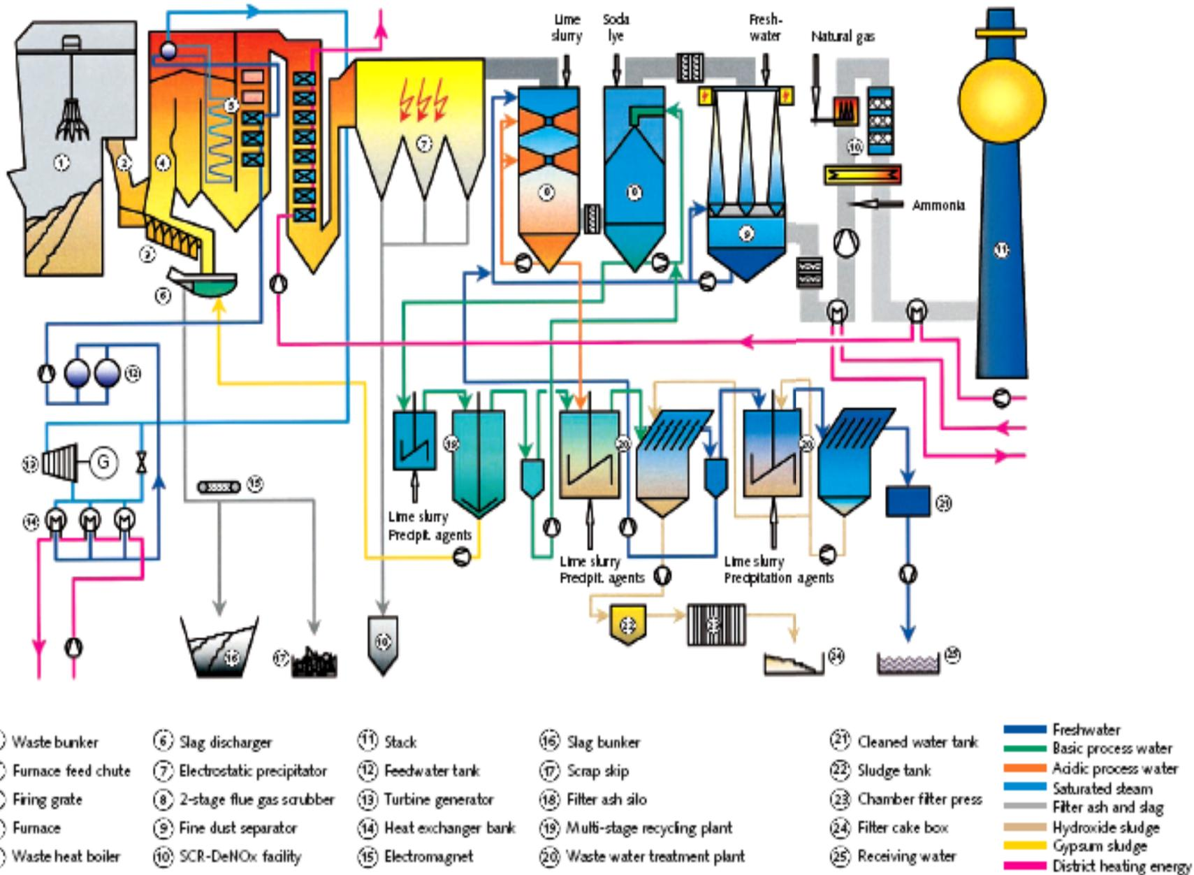
Figure 5: Processing scheme of the WTE facility Spittelau
