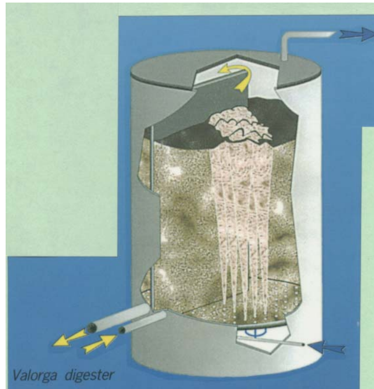
Figure 4. The Valorga Digester
