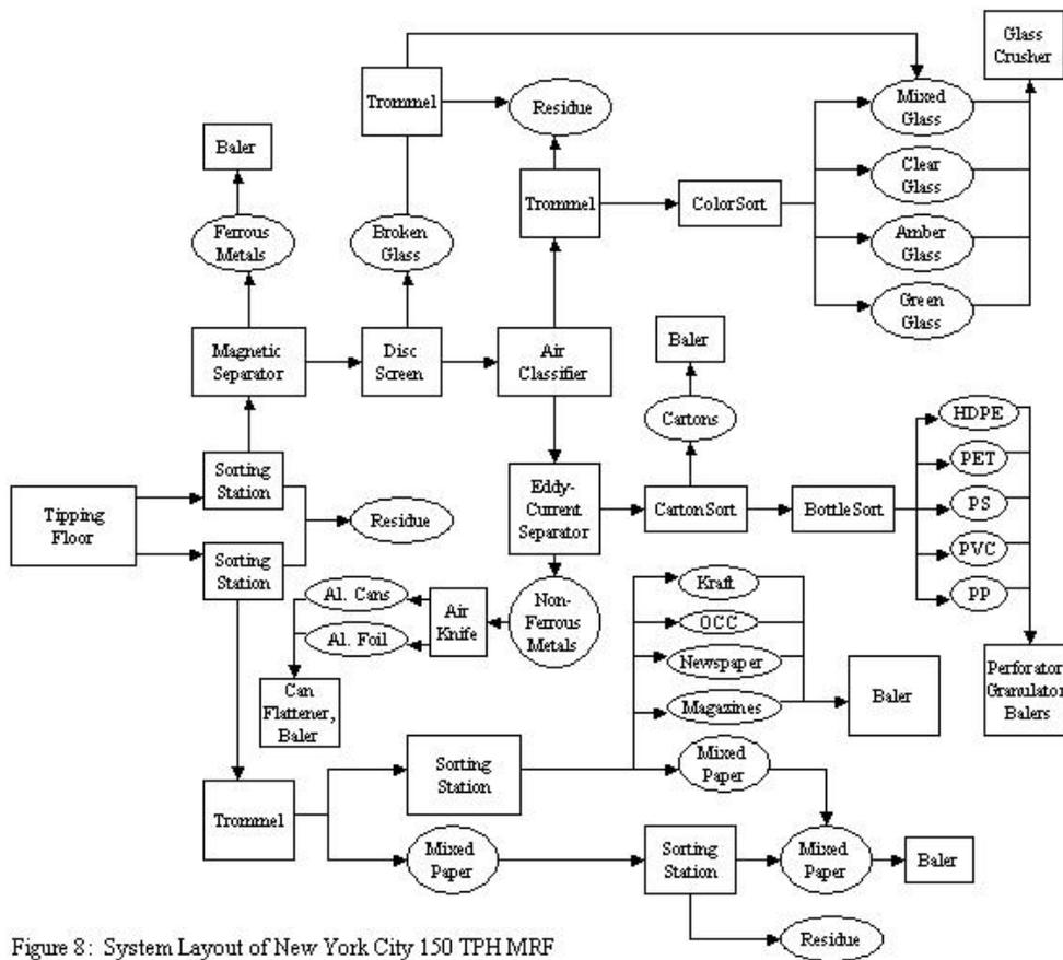
Figure 8: System Layout of New York City 150 TPH MRF
