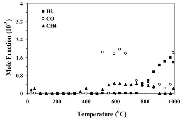
Figure 10. 0% CO<sub>2</sub> Pecan Shell Composite Gas Evolution
