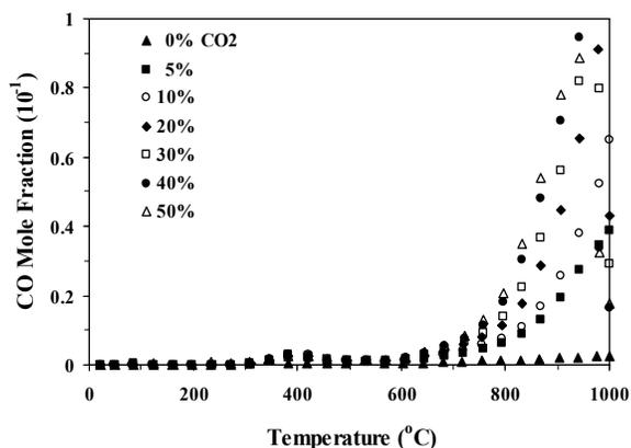
**Figure 20.** CO Evolution from Beachgrass showing CO Enhancement with CO<sub>2</sub> for T > 750°C
