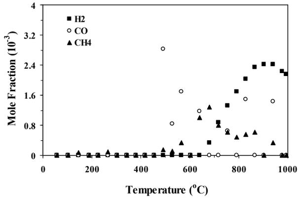
Figure 9. 0% CO<sub>2</sub> Blue Fir Needle Composite Gas Evolution
