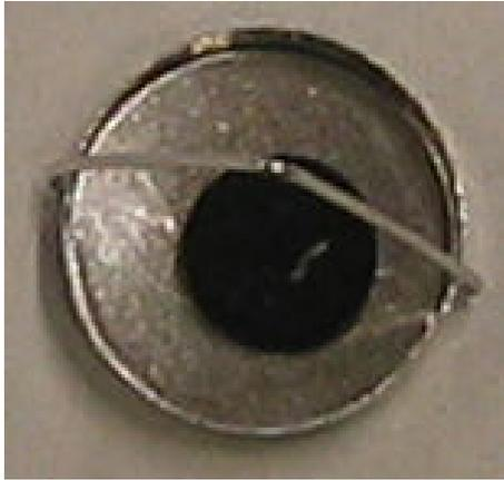
**Figure 3.** Large black char residue from 10% CO<sub>2</sub> spruce steam gasification
