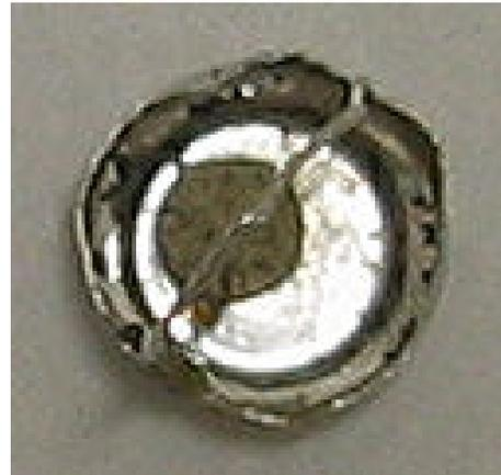
**Figure 6.** Small light mineral residue pancake from 30% CO<sub>2</sub> walnut shells steam gasification
