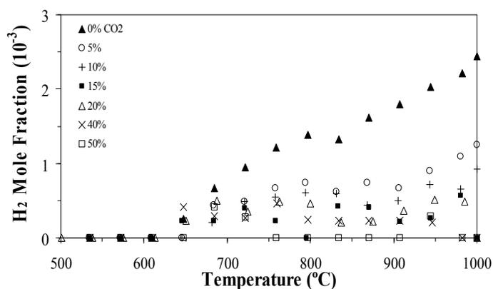
**Figure 21.** H<sub>2</sub> Evolution from Poplar showing H<sub>2</sub> Depression with CO<sub>2</sub> for T > 750°C
