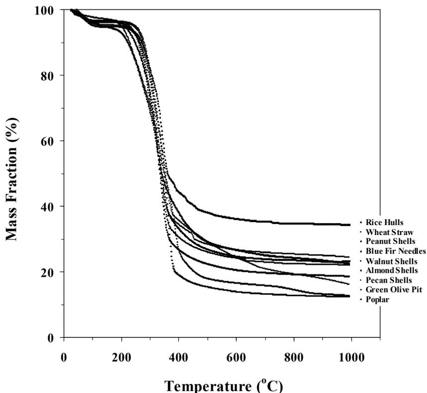
**Figure 2.** Mass decomposition curve for 0% CO<sub>2</sub>
