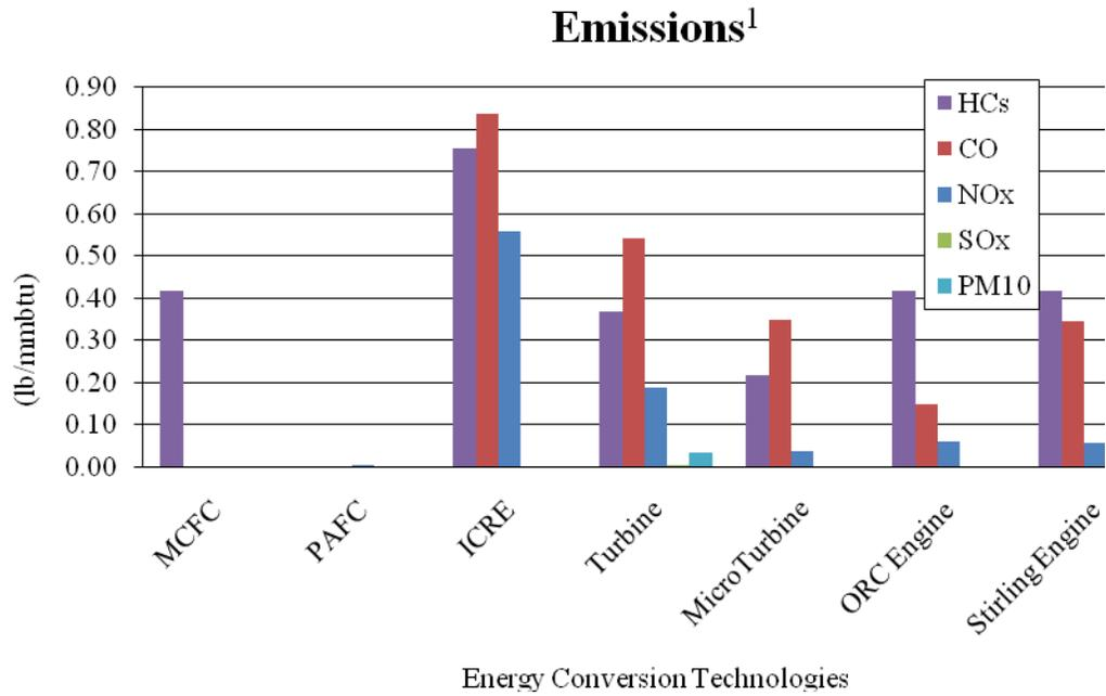
**Figure 4. Emission comparison for various LFGTE technologies**
