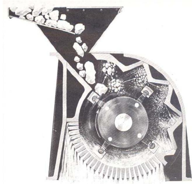
**Figure 2. Operating principle of the high-speed, low-torque hammermill.**
