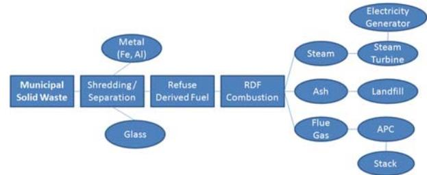
**Fig. 4 Flow diagram of the RDF process**
