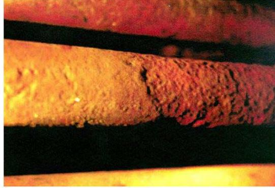
Fig. 1: salt melt corrosion on blank superheater /7/
