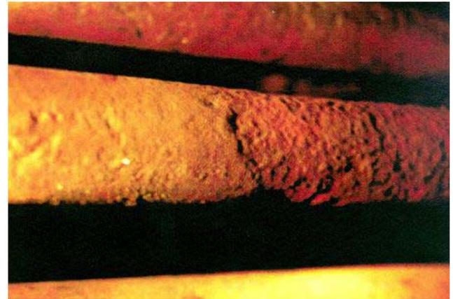
Fig. 3: salt melt corrosion on blank superheater /viii/
