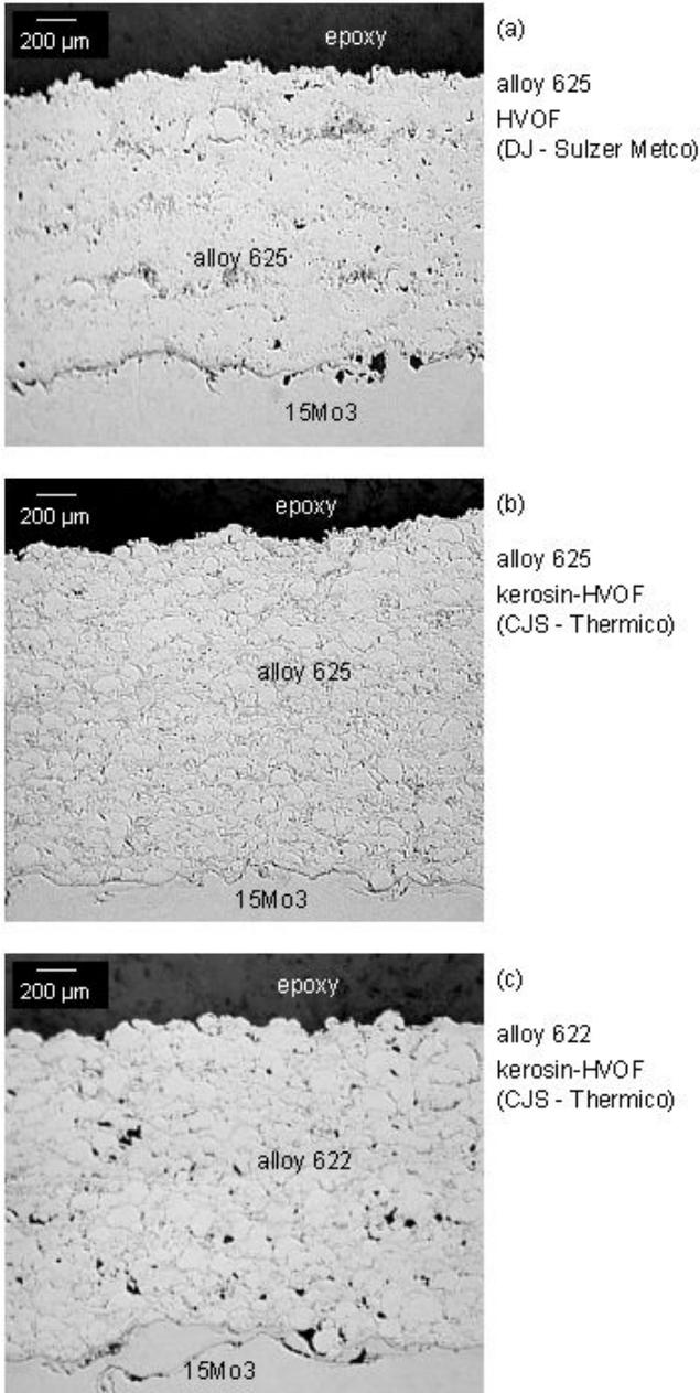
Fig. 4: Nickel base alloys, sprayed by different HVOF processes
