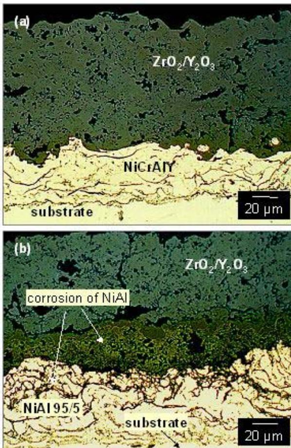
Fig. 2: hot gas test (1000°C, 300h, air);
