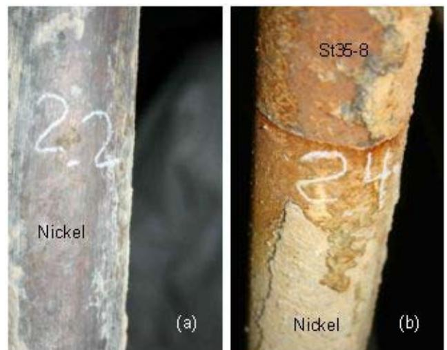
Fig. 7: evaporator tubes (coated with nickel - HVOF) after 4.100 hours of operation (conditions: 285°C/80bar steam; ;
