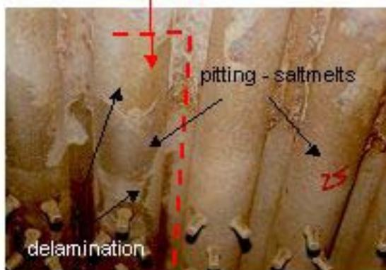
Fig. 6: frontwall (coated with alloy 625 - HVOF) after 7.500 hours of operation (conditions: 240°C/40bar steam; 850°C fluegas), /x/
