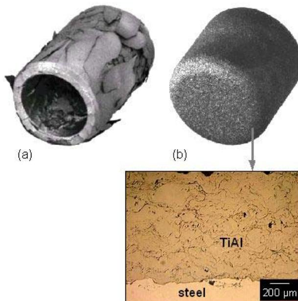
Fig. 1: hot gas corrosion of steel PK925 (X10CrAl18) in reduced atmosphere (Ar-5%H<sub>2</sub>-1%H<sub>2</sub>S);
