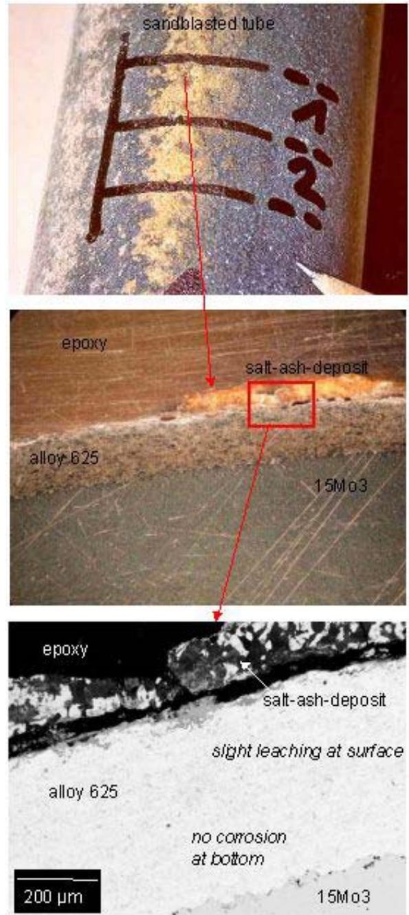
Fig. 5: pre-superheater (coated with alloy 625 - HVOF) after 7.500 hours of operation (conditions: 385°C/40bar steam; 400-500°C fluegas), /x/
